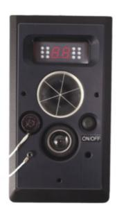
The NTM-10 target module detects the hit and miss and gives a bright flash when hit.
